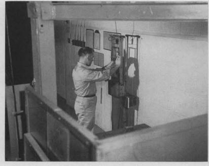
SHOCK TEST DATA is provided by a battery of shock testing machines, from miniature drop towers like the one shown above being adjusted by M. L. Heisler, 1611-3, to two and three-story apparatus. Drop tests can administer shocks as high as 4000 G's!
